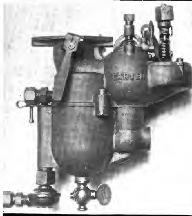
Fig. 7—Other side of the carbureter presenting the remaining lever positions; attention is called to the cock at the bottom for draining out residuum
